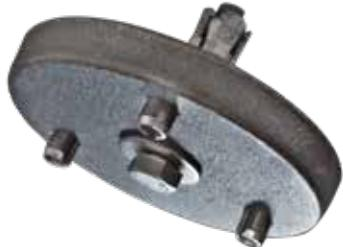
Corrosion protection anode for 4" ZDS motors, manufactured with an alloy suitable for contact with drinking water. It can be easily fit to the lower extremity of ZDS motors to protect them from corrosion in the presence of irregular currents or particularly aggressive waters, greatly increasing the life of the motor components.
