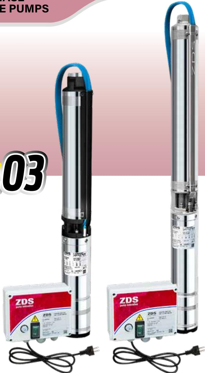
**4" complete submersible pump, made of ZDS hydraulic part, ZDS single-phase PSC oil-cooled O3 motor, supply cable in different lenghts and ZDS CBO electrical start panel (which includes on/off switch, start and run capacitor and overload protector).**
